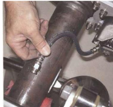
11. Since this brake kit uses floating calipers that move with normal brake wear and operation, it is critical to use a flexible brake line between the caliper and axle housing. A tab should be welded to the housing to support the junction between the flex line and hard line.
