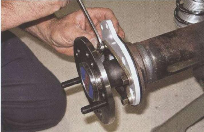
2. Install the base bracket between the spacer and the retainer and secure using the supplied nuts. The ears on the base bracket should be positioned so they will mount the caliper up toward the rear as shown.
