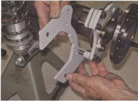
7. Remove rotor and bolt the caliper bracket to the base bracket using the spacer(s) determined in the previous step.
