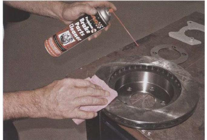
3. Make sure to use a quality brake cleaner and rag to clean the anti-corrosion coating off your brake rotors before installing them. This coating can contaminate brake pads.
