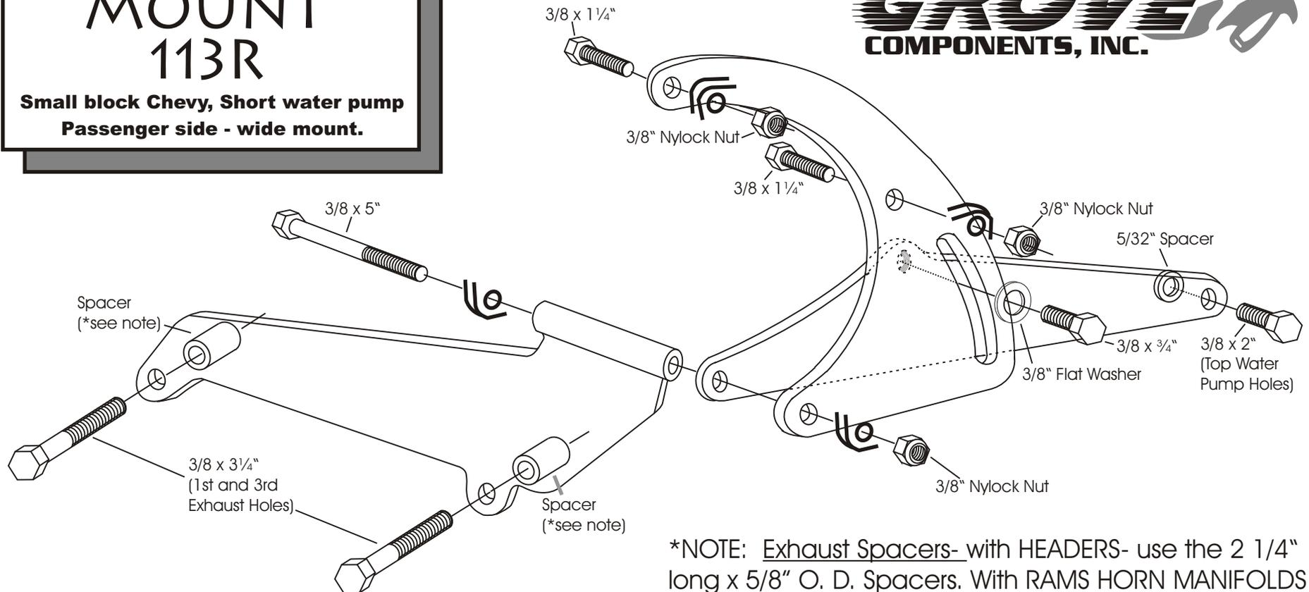
We use a belt length of 60-61" with this mount on installations in our shop. However; this can vary with the diameter of your pulleys.
